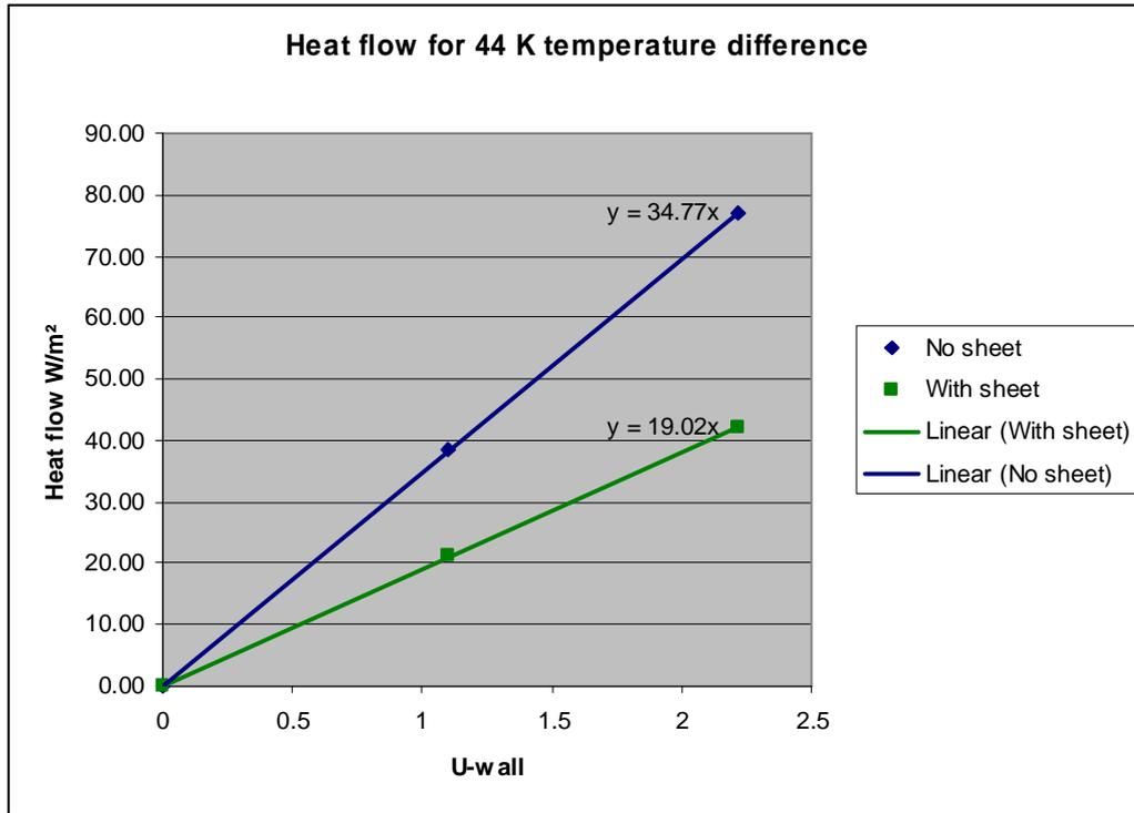
Figure 1 : Heat flow through wall for 44 K temperature difference
